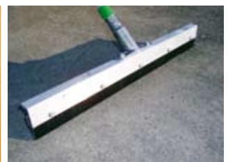
Sealing of a broadcast layer with a straight trowel or "squeegee" blade.
