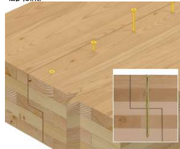
SDCP TIMBER-CP screws installed into a CLT lap joint.
